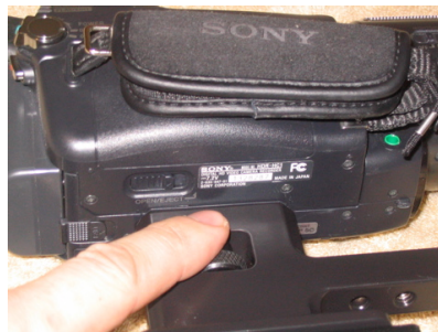
Check to be sure the adapter doesn't block the tape door
