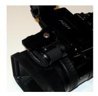
Once original shoe mount is removed, there should be a threaded hole where the old shoe mount was located. Use a fingernail or thumbnail to pull up on the captive screw on the FX1-FLAT and slide it onto the the camcorder. With the manual screwdriver or coin, turn the screw into the threaded hole until it is secure. Do not over tighten the screw.
